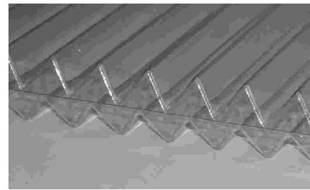
Fig. 1b. Example of the first double layer zigzag-structure manufactured with vacuum form techniques.
