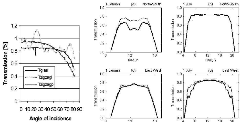
Fig. 3a. Transmission as function of the angle of incidence for incident angles perpendicular (zigzagl) and parallel on the zigzag structure (zigzagg).
