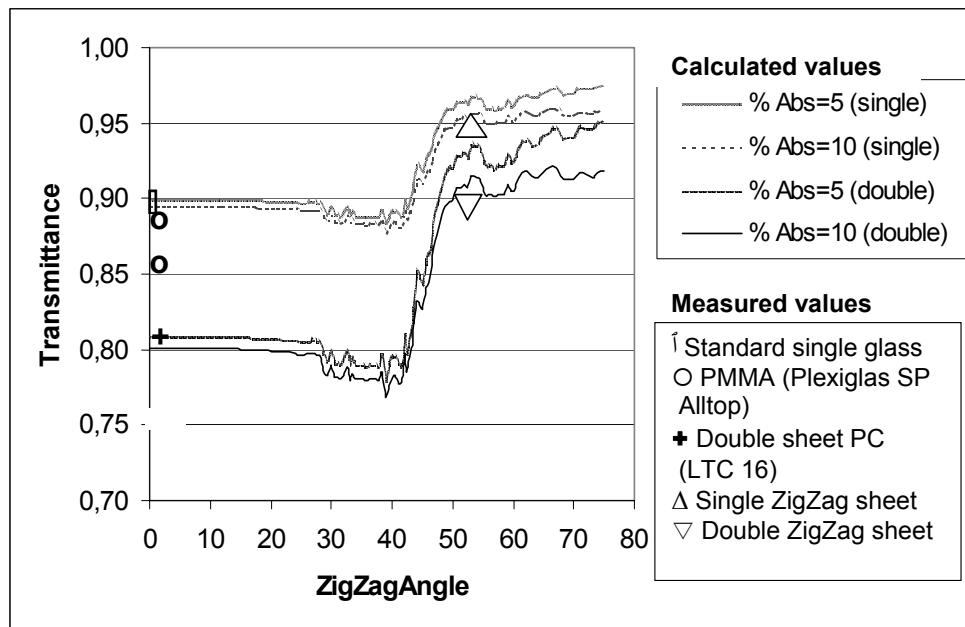
Fig. 2. Overview of the calculated and measured (direct perpendicular) light transmittance of the ZigZag sheet materials (A zero ZigZag angle is a standard sheet material).
